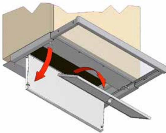
Remove the grease filters by pulling down the two stainless steel hinged lower cover plates at the front side, which covers the grease filters. Pull the two metal grease filters down by the little hook.
